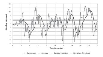
Figure 1: Gyrosope values over time, showing the periodic natural body sway during walking (blue crosses) and the results of the averaging algorithm (dark red). These plots can be seen as different interpretations of the user's trajectory over time.
