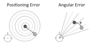
Figure 2: Positioning error (left) and angular error (right). In both figures, the blue circle represents the true location of the sound source and the green circle represents the location of the source as marked by the user.
