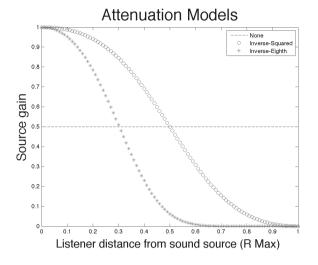
Figure 1: Attenuation Models used in each experimental condition.
