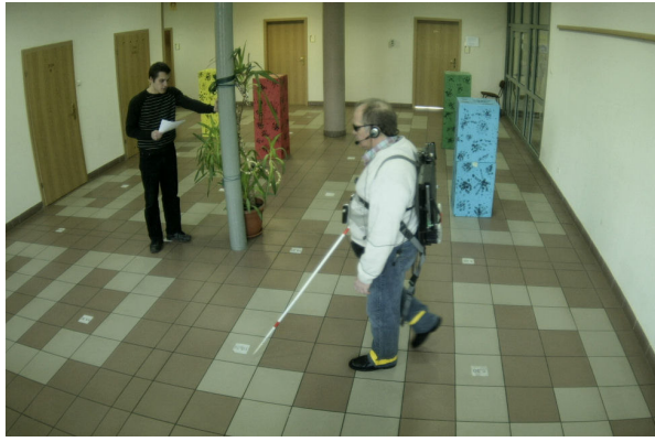
Fig. 2 Navigational trials were automatically recorded. Markings on the participants' pant legs and on the floor allowed precise path reconstruction.
